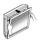
2. Pull out the both links of lower part of front panel, as described in the below picture.
